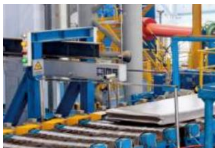
Rough roll mill exit IMS crown tester
