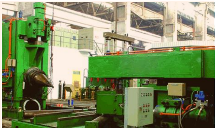
5000mm radial and axial CNC ring rolling machine
