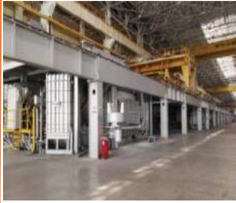
Hydraulic tilting gas heating furnace
